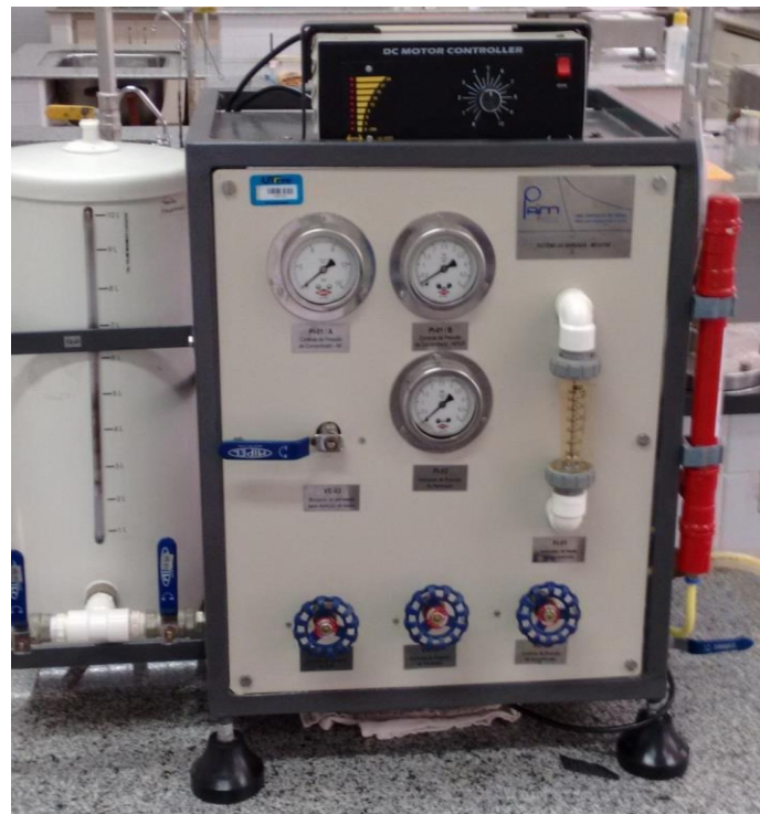
Figure 2 – Picture of the micro and ultrafiltration bed system
