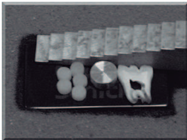
Figure 1 - Aluminum step wedge, resins, lead and tooth on sensor CCD CDR- Schick Technologies. Piracicaba-SP (Brazil), 2001
