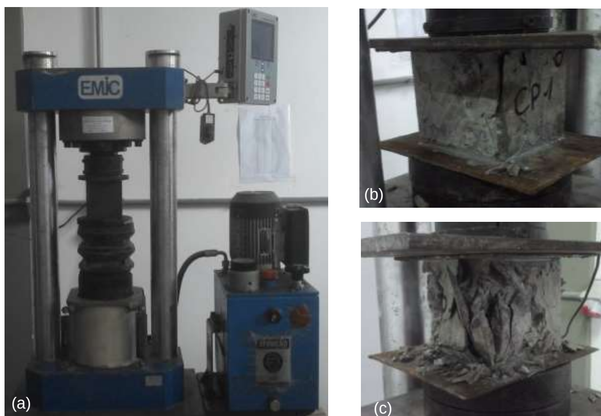
Figure 2 (a) Uniaxial testing machine Emic / PC150C, (b and c) view of tested sample at times t_i e t_f .
